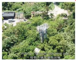
RBS conditions are live streamed through the drone camera for inspection by maintenance personnel in real time
