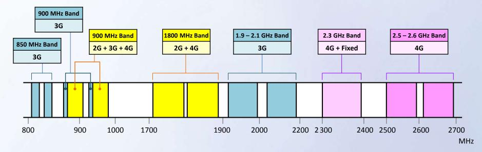
Currently, public mobile services are operating below sub-6 GHz bands (1 GHz = 1000 MHz). Given the favourable radio propagation characteristics, territory-wide coverage with high network capacity can be achieved by transmitting at relatively lower power and reusing frequencies
