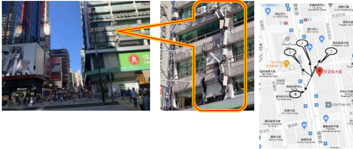
Figure I-5: Photo of Test Site 7 and diagram illustrating the directions of the boresight of the RBS antennas represented with arrows and the measurement points.
