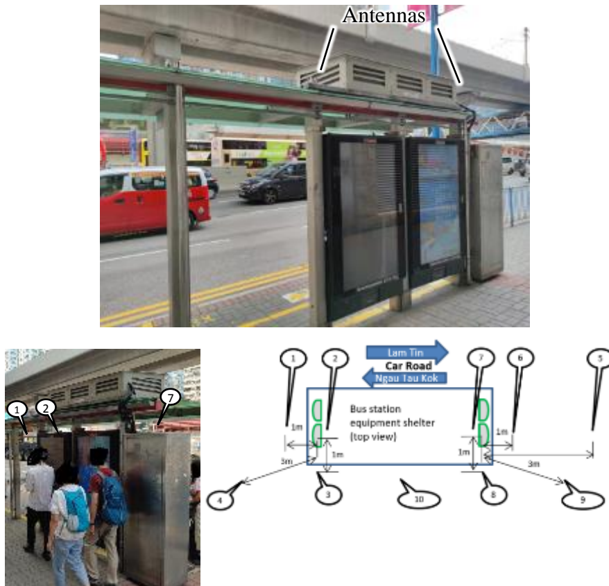
Figure I-2: Photo of Test Site 4 and the measurement points.
