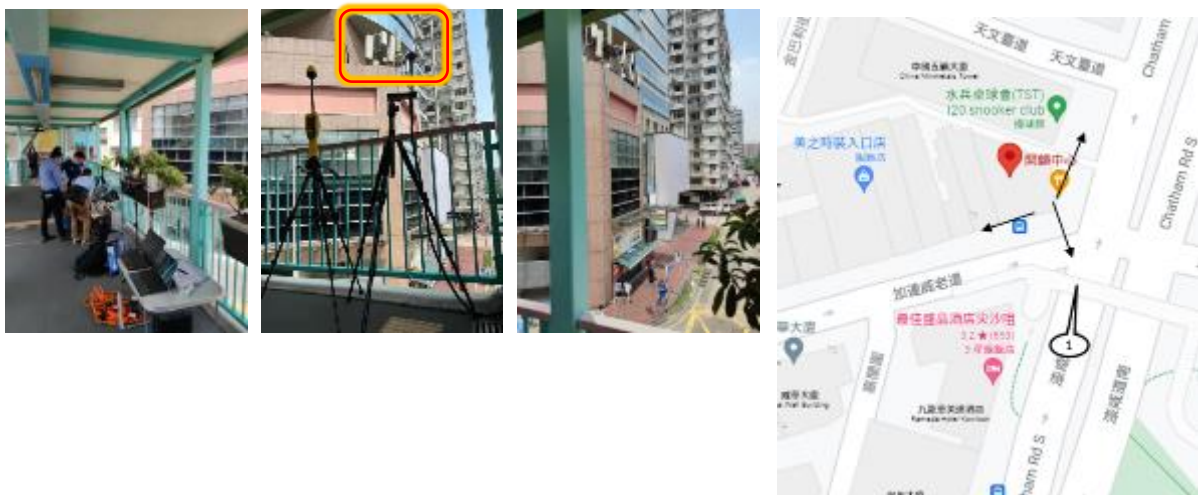
Figure I-3: Photo of Test Site 5 and diagram illustrating the directions of the boresight of the RBS antennas represented with arrows and the measurement points.
