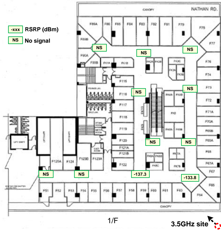
Figure 16. 3.5GHz indoor penetration test result – 1/F
