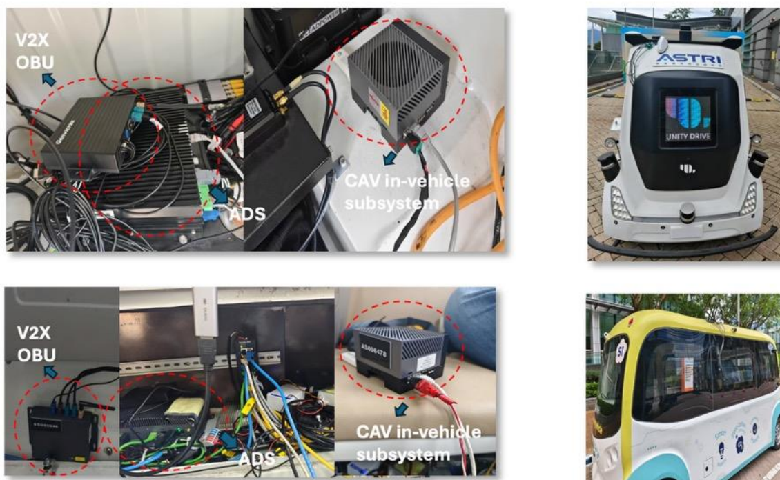
Figure 17 In-Vehicle V2X Setup
