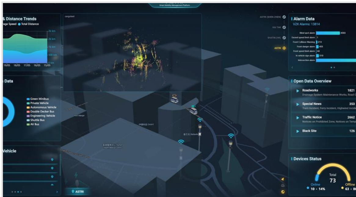
Figure 19 Real-Time Vehicle-Side Point Cloud Transmission via V2X
